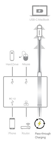
The Kanex USB-C to Gigabit Ethernet Hub with Power Delivery gives you instant high speed Ethernet access. It adds an extra high speed USB port to your MacBook to connect peripherals and charges it simultaneously with power delivery. With data transfer speeds of up to 5 Gbps and a compact portable design, this versatile adapter will become an essential tool to your everyday workstation.
